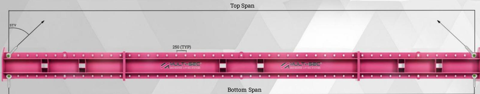
In spreader beam configuration, the Multi-Sec Multi-Point Lifting Beam can be used in a **3m, 6m, 3m + 6m** (max 9m span) or **3m+6m+3m** (max 12m span) configurations. Angled top slings connect to top lifting points to match bottom spans at two positions. This allows for a single beam set up to achieve multiple lifting spans depending on the load being lifted. A spreader configuration is suitable for a standard 2 point lift.
